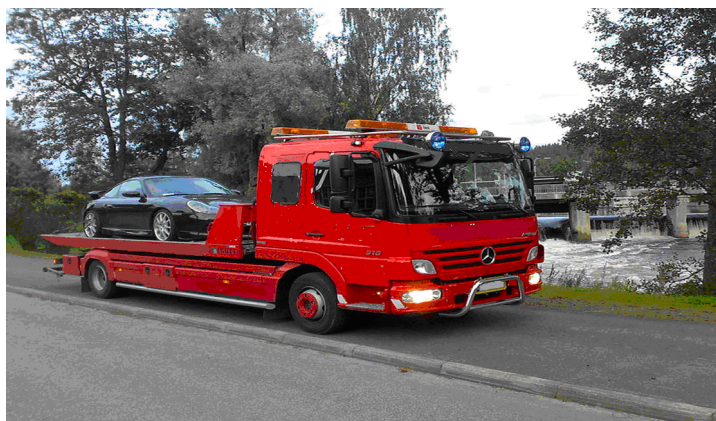
TOW – Tow Truck. These vehicles are designed to tow a vehicle and have a rear lifting device.
