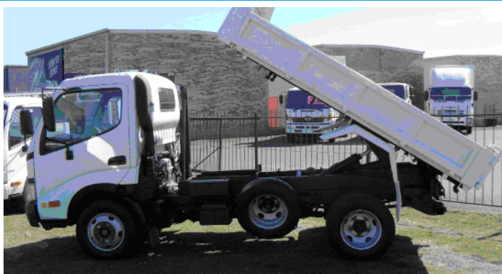
TPR – Tipper. This vehicle has a separate tipping body.
